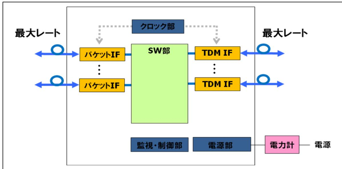
【 $P_{idle}$ 測定時の構成例(最小実装の最小パス構成)】
