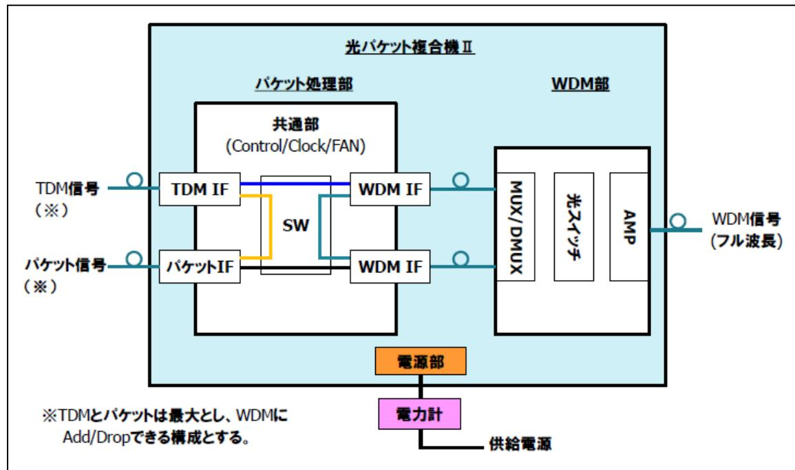
【 $P_{idle}$ 測定時の構成例(最小実装の最小パス構成)】
