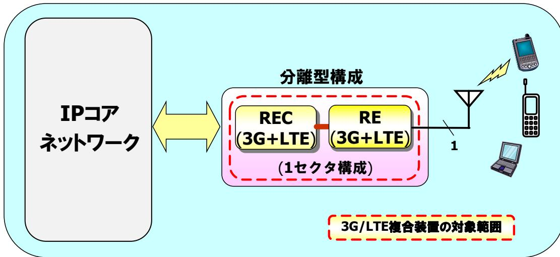
LTE:Long Term Evolution REC:Radio Equipment Control RE:Radio Equipment
