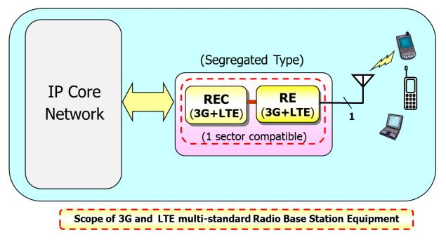
REC: Radio Equipment Control RE: Radio Equipment
