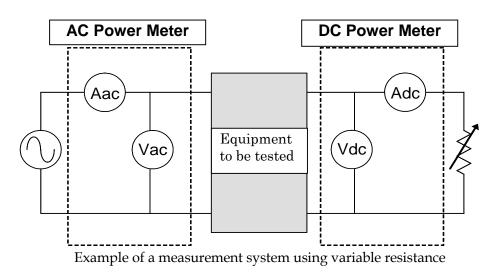
Using variable resistance, measure conversion efficiencies  $\eta_{100}$ ,  $\eta_{75}$ ,  $\eta_{50}$  and  $\eta_{25}$  at nameplate currents of 100%, 75%, 50%, and 25%, respectively, and seek the average value  $\eta$ .
