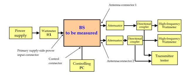
**%1** An ammeter or voltmeter may be used in place of a wattmeter
