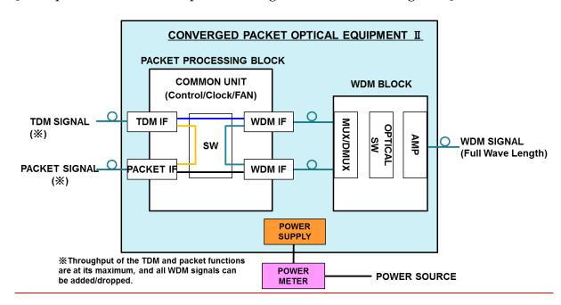
[Example of minimum component and path configuration for measuring Pidle]
