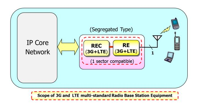
REC: Radio Equipment Control RE: Radio Equipment
