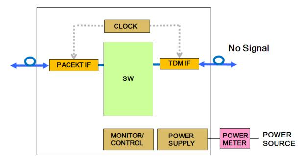
[Example of minimum component and path configuration for measuring P<sub>idle</sub>]
