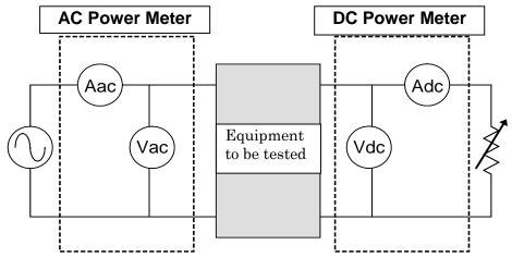
Example of a measurement system using variable resistance
