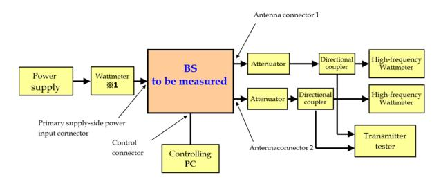
**\*1** An ammeter or voltmeter may be used in place of a wattmeter
