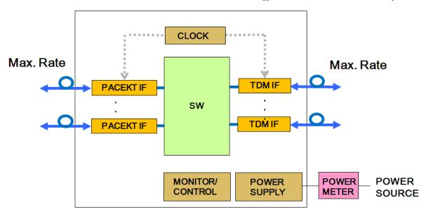
[Example of minimum component and path configuration for measuring Pidle]
