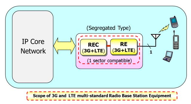
REC: Radio Equipment Control RE: Radio Equipment
