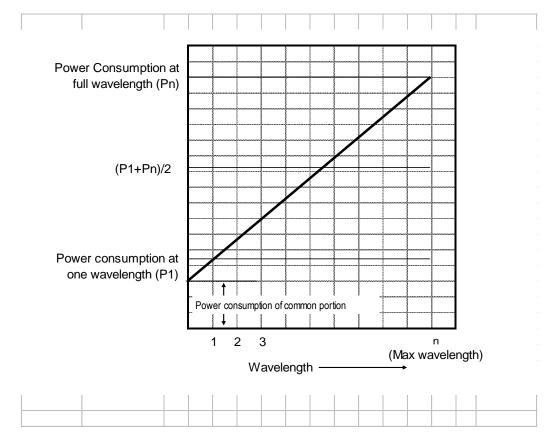
Given that equipment configuration differs by vender, it is preferable to use the following parameters, which rely largely on power consumption and enable stipulation through external interface.
