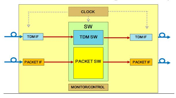
Model II: Configuration where some TDM signals are converted into packets and switched via the packet switch, or some packet signals are depacketed and switched via the TDM switch.
