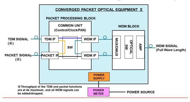
[Example of minimum component and path configuration for measuring P<sub>idle</sub>]
