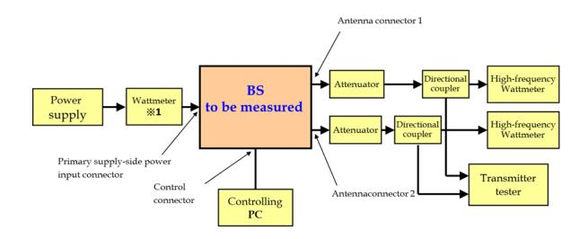
X1 An ammeter or voltmeter may be used in place of a wattmeter
